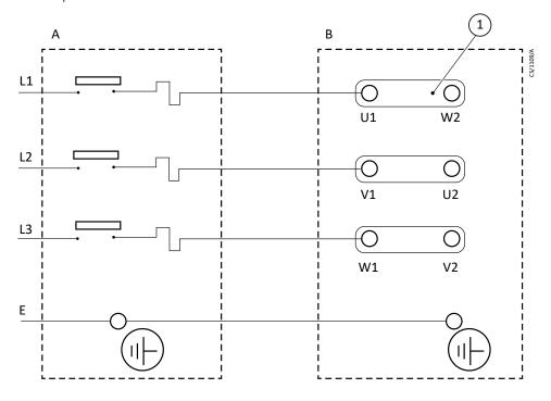
The above three-phase electrical connections are for RV3 and RV5
